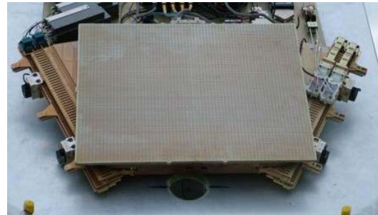
ERA G3 Tx/Rx antenna for trains/airplanes Electromechanical elevation scan 20o to 70o scan Low cost injection moulded and metallised plastic
