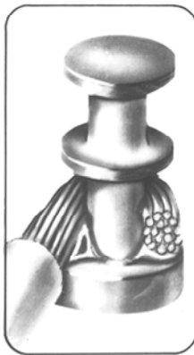
Unacceptable Insufficient solder
