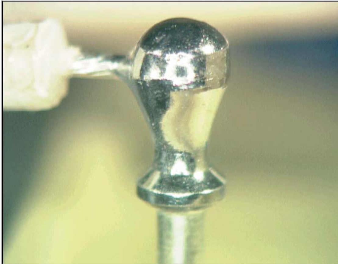
Figure 10-1: High voltage connection
