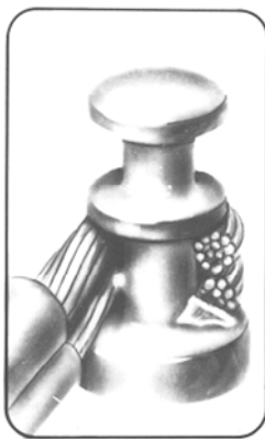
Unacceptable Insufficient solder
