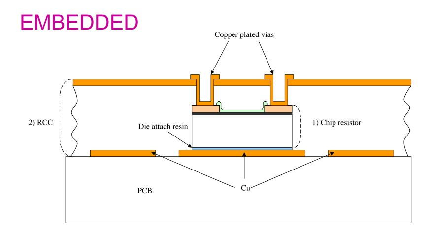
2) RCC: Resin Coated Copper (or prepeg + copper)
