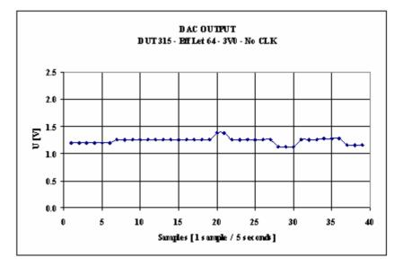
DAC output changes in the G3AD ASIC, error correction disabled
