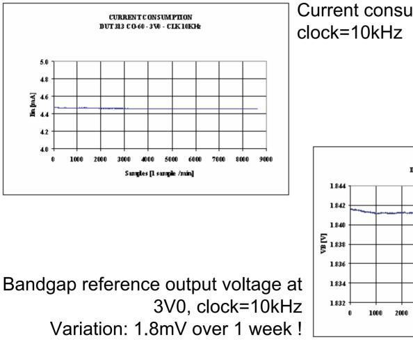
Current consumption at 3V0, clock=10kHz
