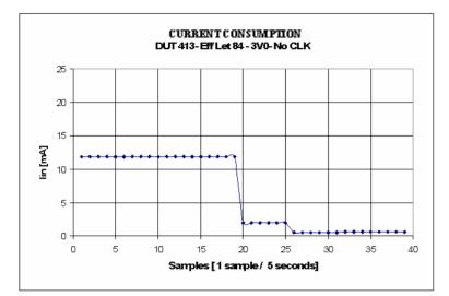
**SEU** in power register at Let84, 3V6, clock=0Hz (no error correction)
