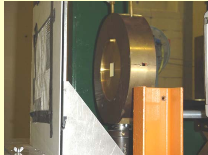
KVI degrader from 184 MeV primary energy down to 60 MeV
