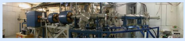
Time-of-flight spectrometer used to determine energies with and without target foils
