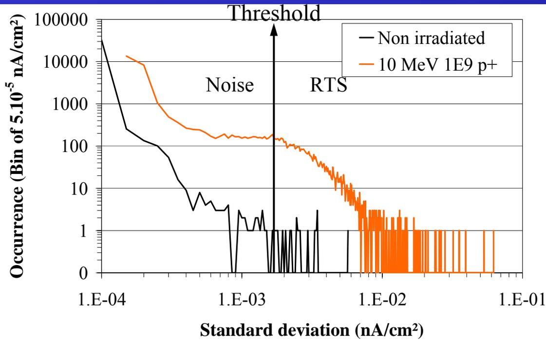
Standard deviation histogram of 32,760 pixels, 5,000 measurements  $T_i = 20\text{s}$ ,  $-10^\circ\text{C}$
