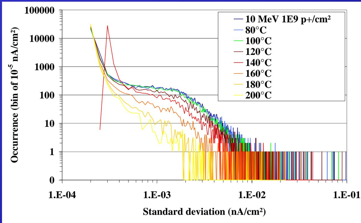
Standard deviation histogram evolution after different annealing temperatures,  $T_i = 20s$ ,  $-10^\circ C$  32,760 pixels
