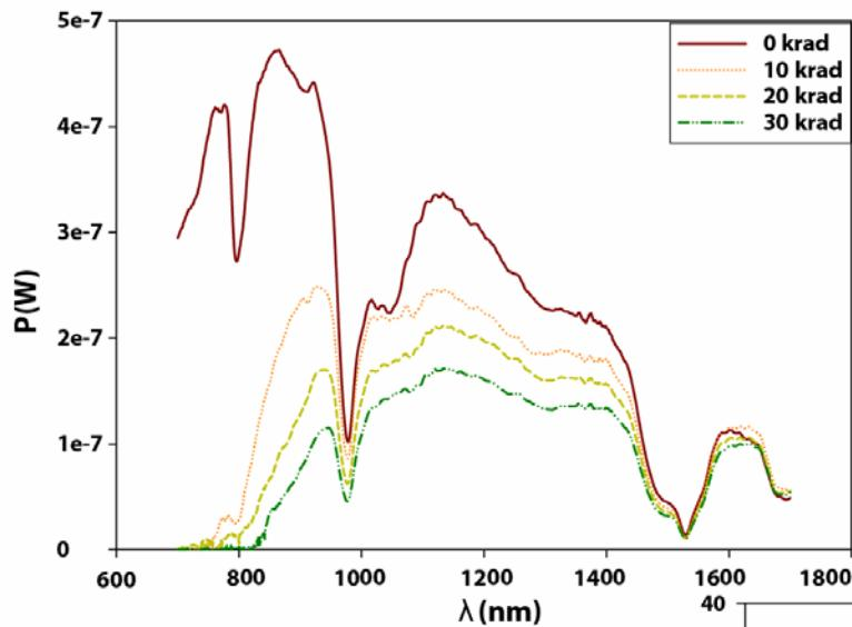
Transmitted power spectra at each dose deposit step.
