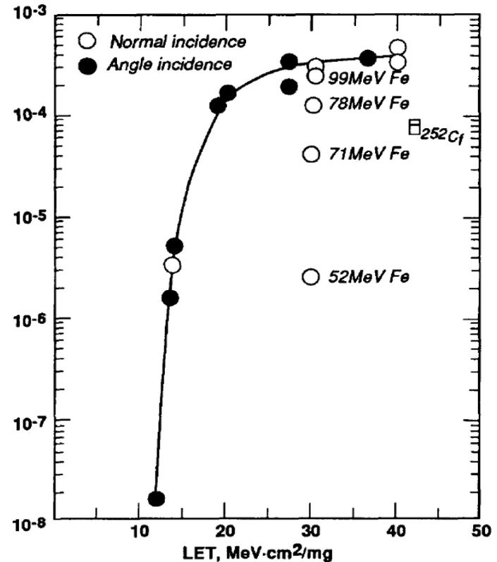
•Levinson showed that ion range influenced SEL cross section [Single Event Latchup (SEL) in IDT 7187 SRAMs-dependence on ion penetration depth," RADECS 93 (1993)]
