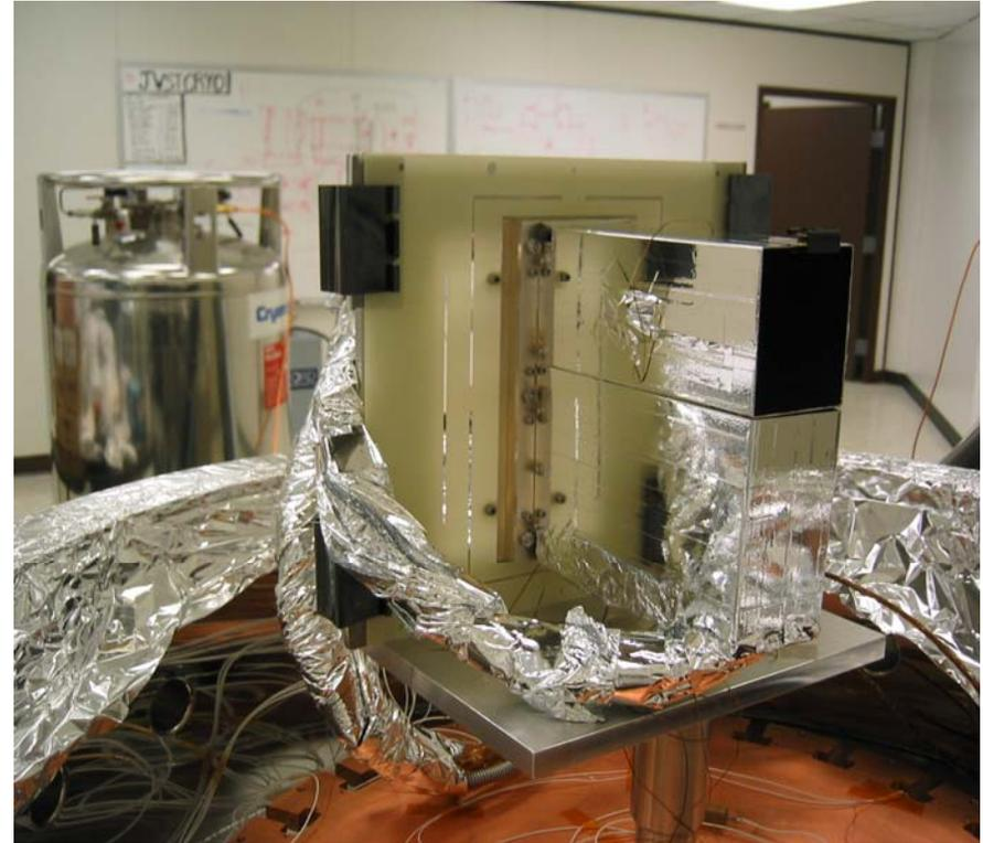
Apparatus used by BATC to test MOSFETs for enhanced Gate Rupture susceptibility at cryogenic Temperature.
