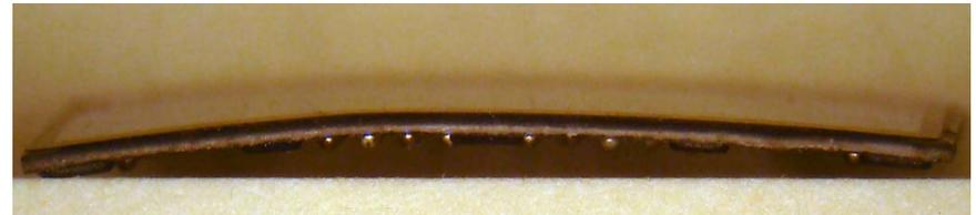
Note that the bowing in the middle has pulled up solder balls off of the carrier. Where does this stress come from? Will it be a general feature in deep submicron feature size CMOS?
