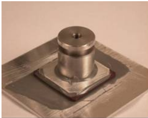
Package prepared to 2° pull-out
