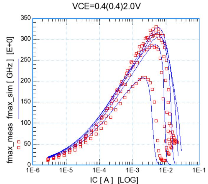
SiGe HBT  $f_{\text{Max}}$  versus  $I_{\text{collector}}$
