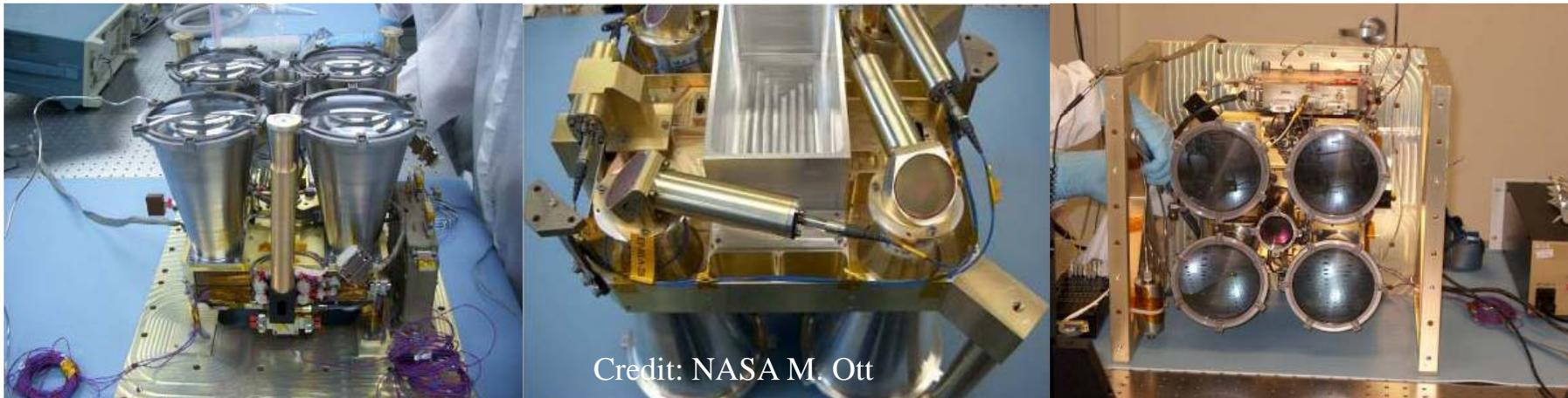
The Mercury Laser Altimeter consisted of four telescopes with fiber coupled from each to four individual detectors
