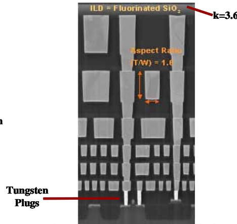
**Intel 0.13µm Process (Cu)**
