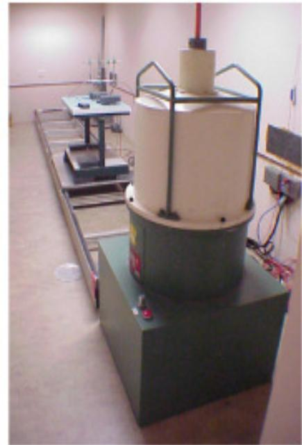
The nominal activity is 2000 Ci for Total Dose Testing but the present activity is around 1465 Ci (Nov 10<sup>th</sup> 2009) which permits dose rates between 0.7 and 50 Rads/min (0.007 and 0.5 Gy/min). At 1m the dose rate is 28 rads/min
