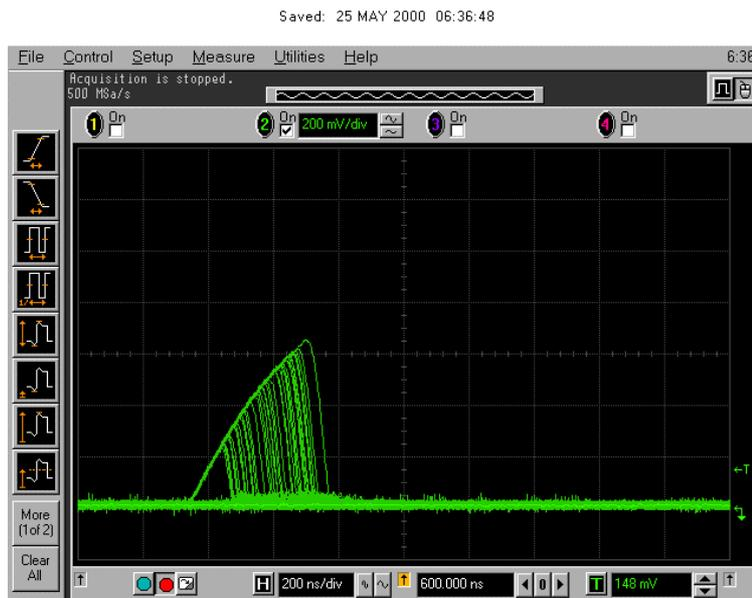
FIGURE 5.1.3 - MOT SN206, 12V BIAS, AR WITH LET.EFF = 28,2 MEV/MG/CM2
