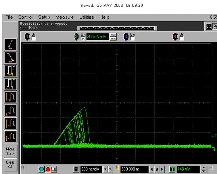
FIGURE 5.2.2 - MOT SN214, 12V BIAS, AR WITH LET.EFF = 28,2 MEV/MG/CM2
