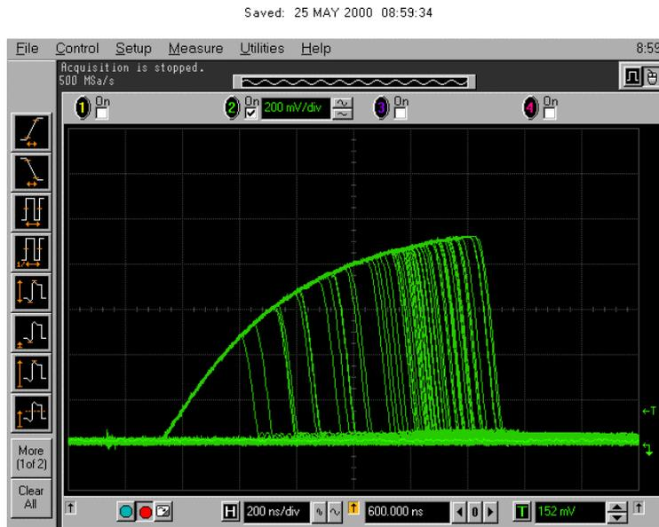
FIGURE 5.2.4 - MOT SN214, 12V BIAS, XE WITH LET.EFF = 111,8 MEV/MG/CM2
