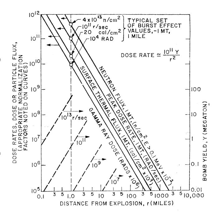
FIGURE 4.1 - NOMINAL RADIATION LEVELS FROM NUCLEAR EXPLOSIVES IN SPACE
