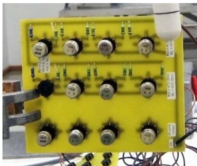
**Figure 9: Test sample mounted on the Radiation Test Board**
