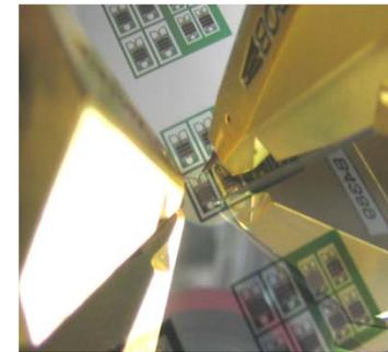
S-parameter test of RF MEMS
