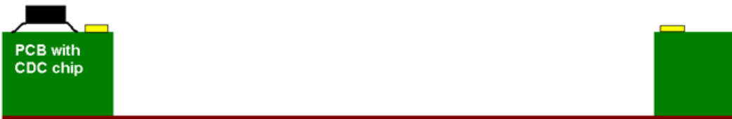
Kapton tape for mounting ES chip onto PCB with CDC chip
