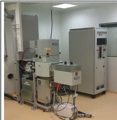
DRIE for hard/dielectric materials (quartz, GaPO 4 , SiC, ..)
