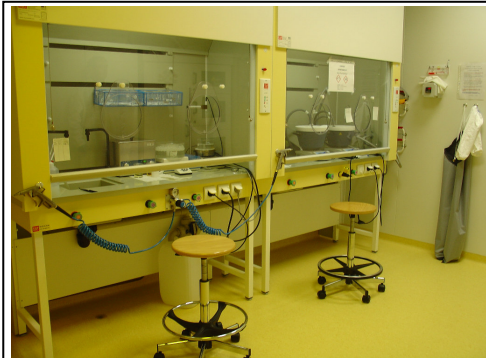
Surface preparation and Quartz Etching Hoods
