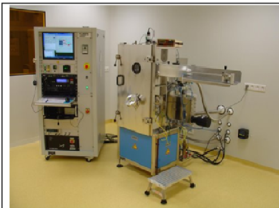
Metallic thin film deposition by evaporation (Ti, Cr, Au,..)
