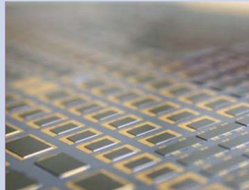
RF Mems with 50 μm silicon cap (polymer bonding)
