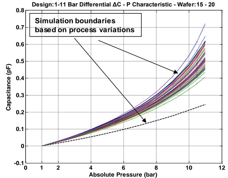
Sensor: 1-11 Bar Differential / Temp Range: -10 to 80 °C (20 samples)
