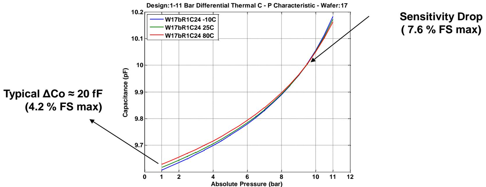
Temperature related offset drifts in  $C_{sense}$  are partly compensated with a reference capacitor using differential electronics architecture
