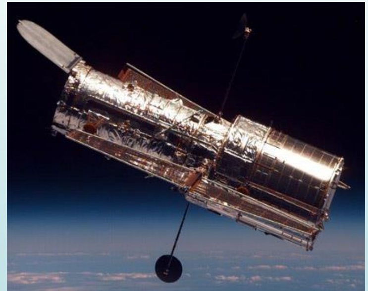
The Hubble Space Telescope (HST) is a 2.4-m (7.9-ft) aperture space telescope. It was carried into low Earth orbit by a Space Shuttle in 1990, and it remains in operation.
