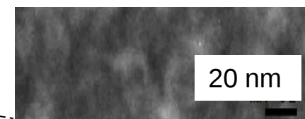
Pitting after 3000 h RF life test @ T_{ch} > 300\text{ }^{\circ}\text{C}
