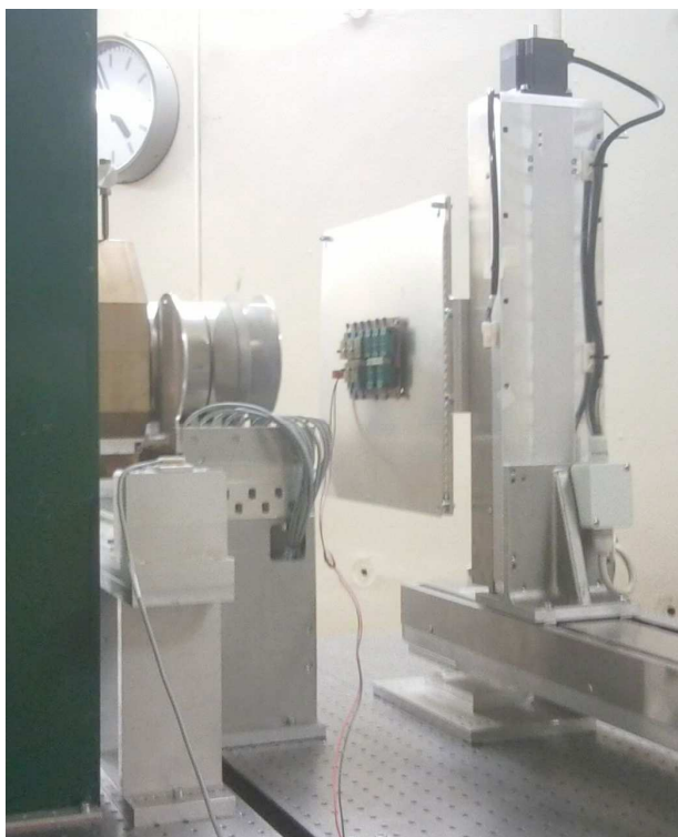
Figure 6: samples installed for irradiation
