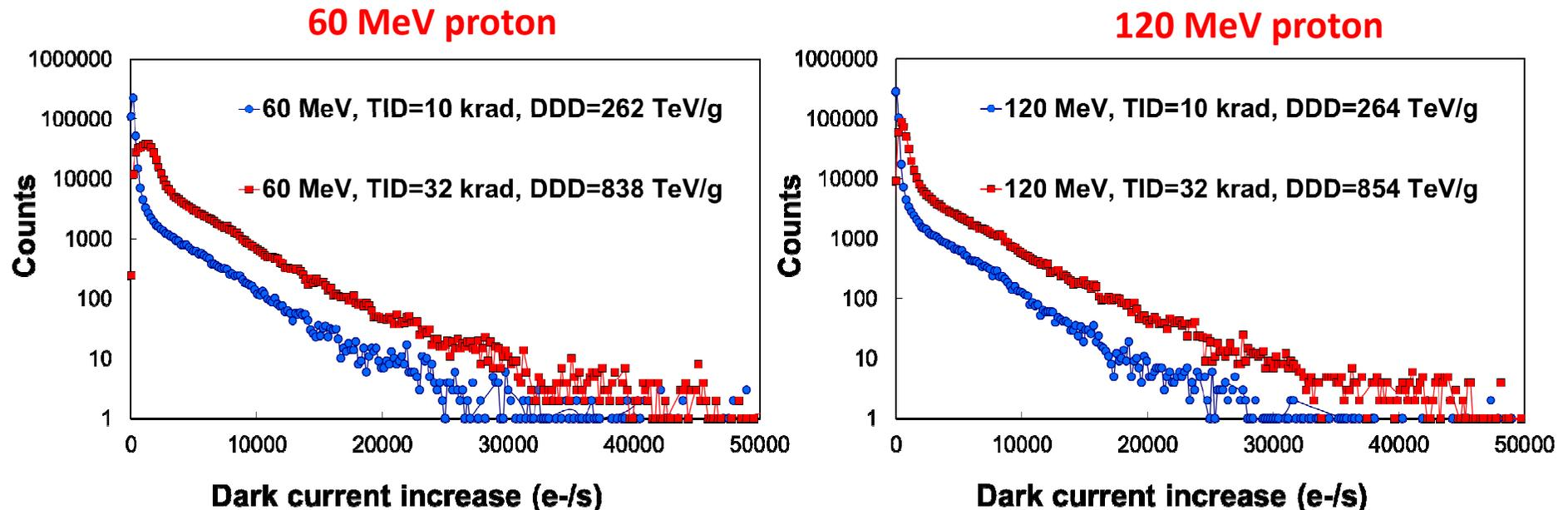
⇒ **Mean dark current increase and the number of hot pixels both increase with the displacement damage dose (DDD)**
