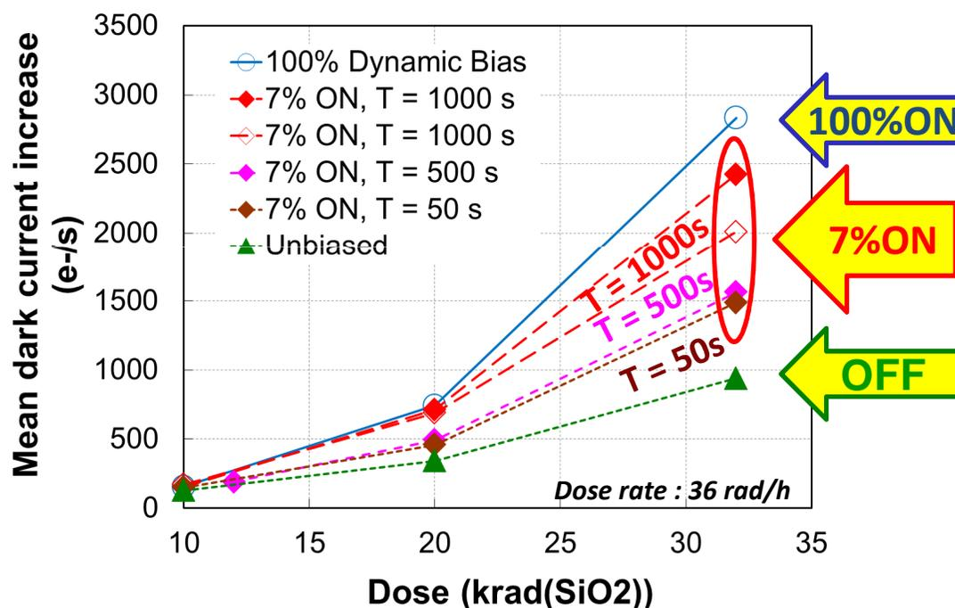
⇒ 7%ON degradation is **bounded** between unbiased and 100%ON degradation
