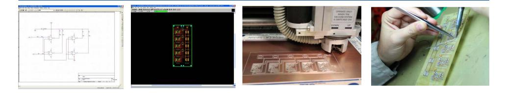
We cover all the processes: circuit design, PCB design layout, PCB manufacturing, assembly and verification, installing adequate low insertion force sockets & SW test development for parameters monitoring
