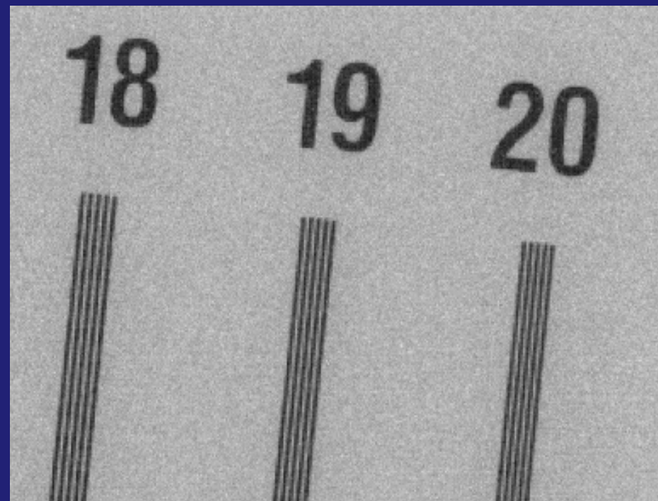
Scint-X scintillator (20um pitch)
