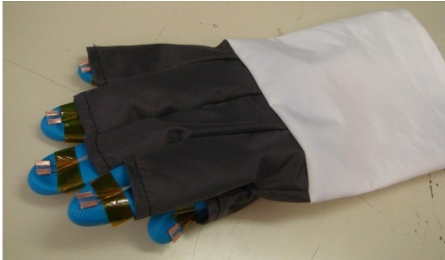
Radiation sensors are integrated onto a space glove
