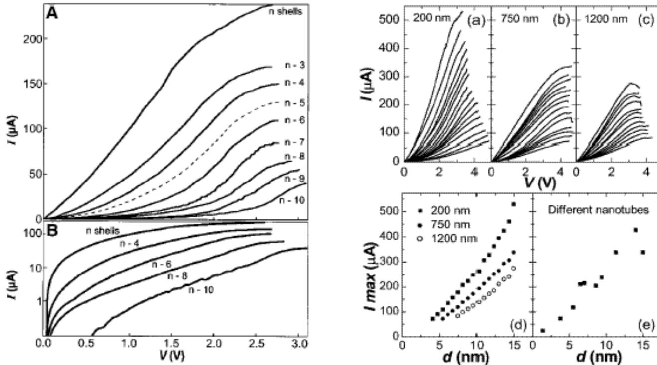
**Current through NT depends on length and diameter of MWNTs**
