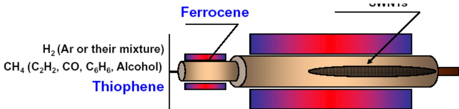
Deposition of catalyst is not required
