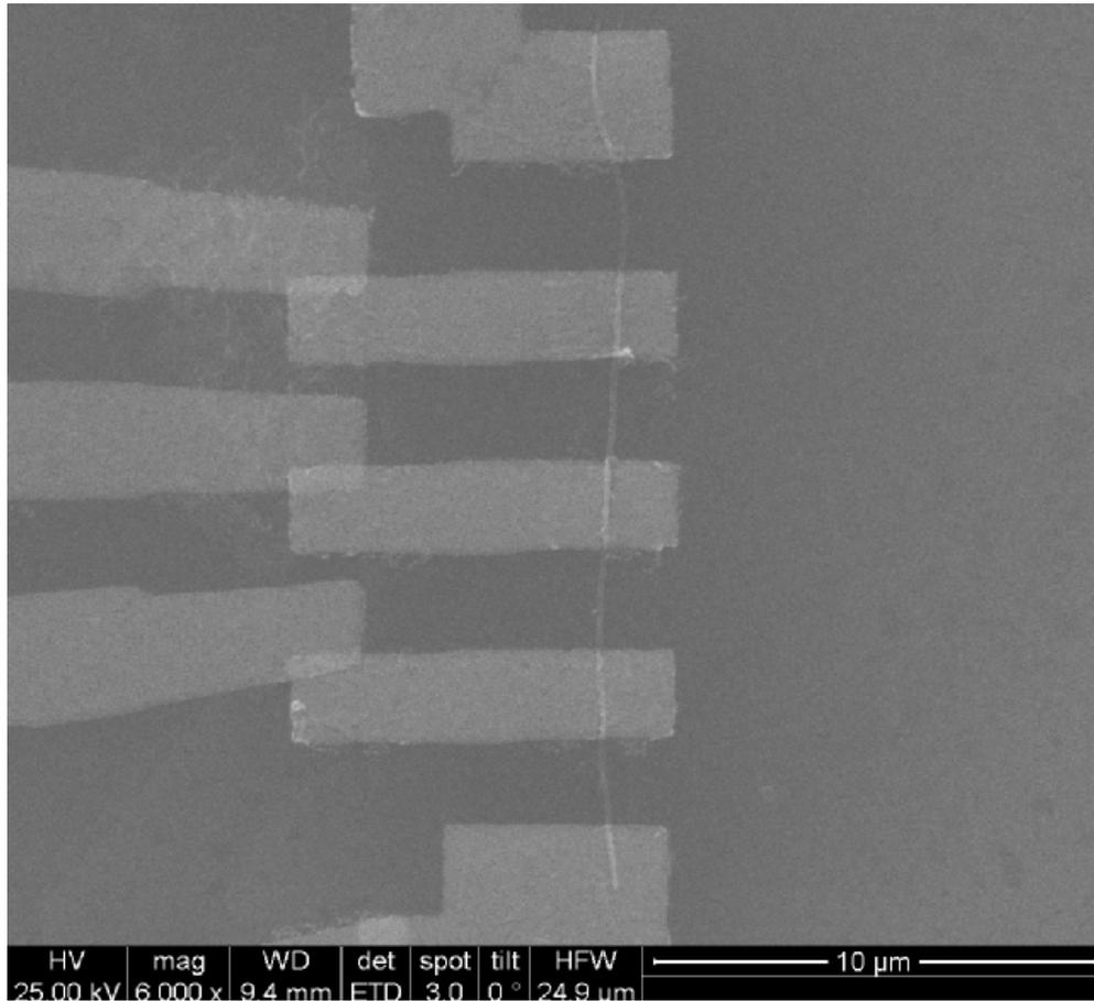
Resistance is  $\sim 4 \text{ k}\Omega/\mu\text{m}$  and the current through the NT is  $\sim 0.5 \text{ mA}$
