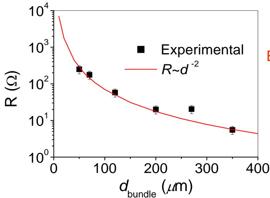
Extrapolated  $R$  for a single NT is  $250 \text{ k}\Omega/\mu\text{m}$
