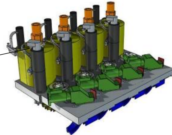
Analysis subsystem concept (11 x 8 x 6,5 cm 3 )
