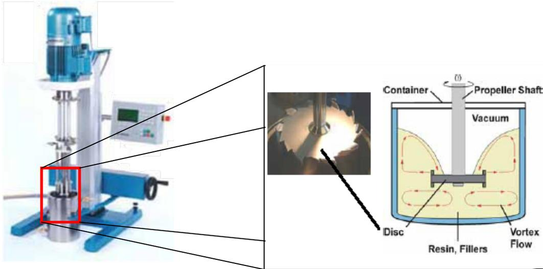
Dispersion of MWCNT into the resin system using Dissolver Technology
