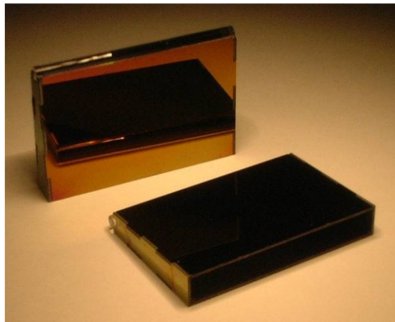
Precision silicon trailing edge box structures
