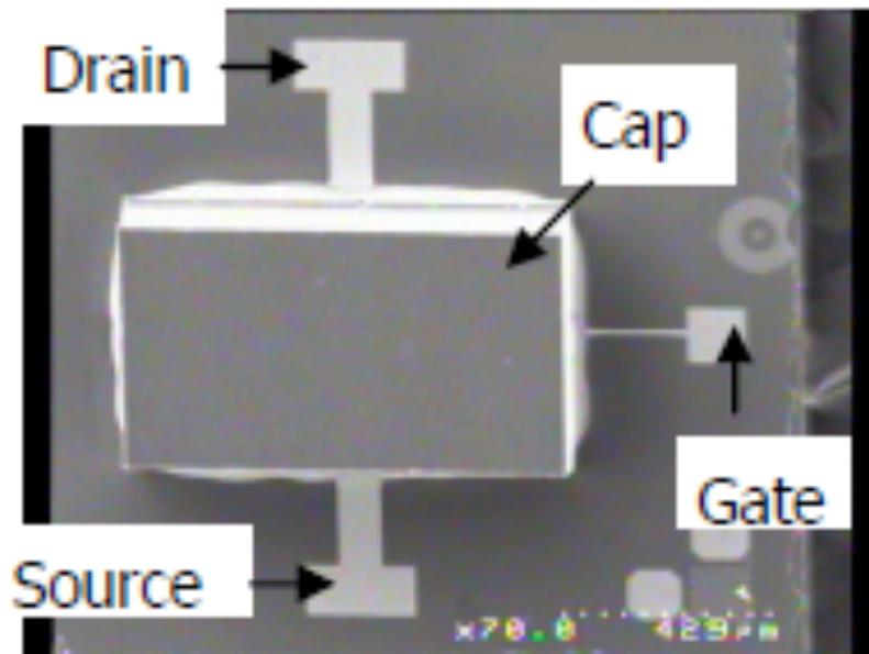
90 Volts applied.  $V_p$  is 81 Volts.
