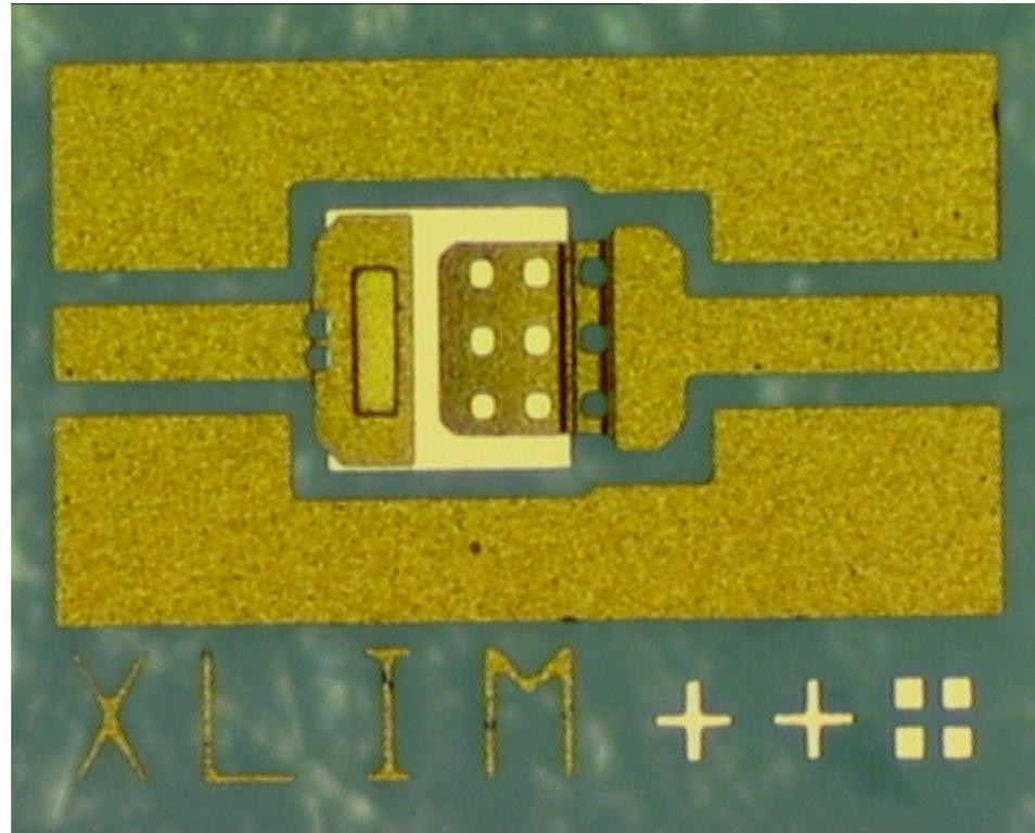
Cantilever beam, insensitive to temperature up to 80°C
