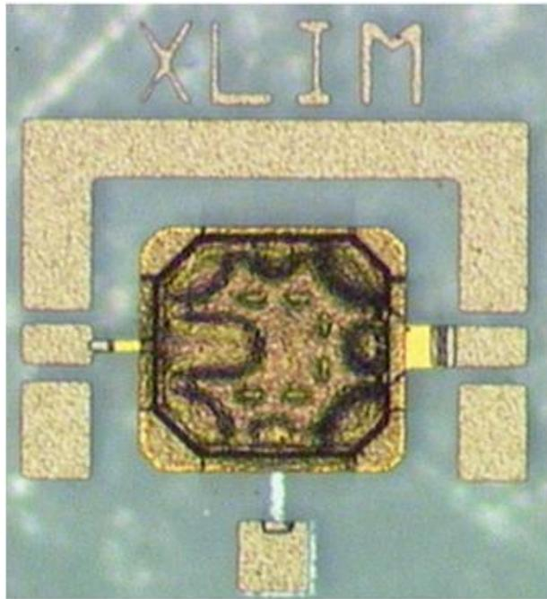
30 Volts applied.  $V_p$  is 24 Volts.
