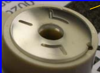
Rotary valve to control the fluid over the chip
