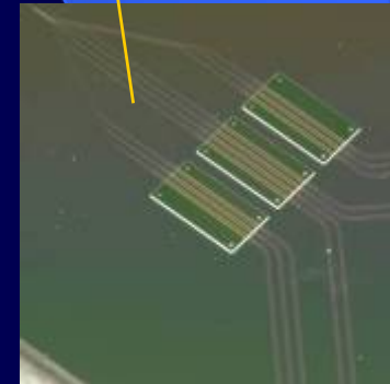
Waveguides to excite the attached antibodies
