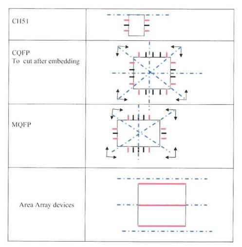
To check absence of damage of the PCB
