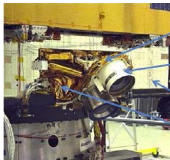
Mobile plate Ion thrusters ( x2 ) Satellite structure Multi-layer insulation
