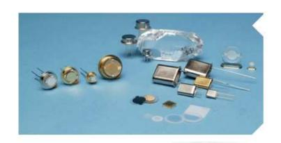
=> Hybrid Crystal (Crystal, thermistors, resistors...)
