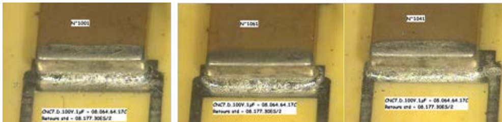
Sn60-Pb40 soldering paste reflow method hot plate / vapor phase / iron hand)
