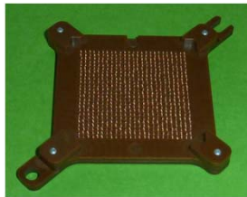
Pressure connector: Hypertac interposer
