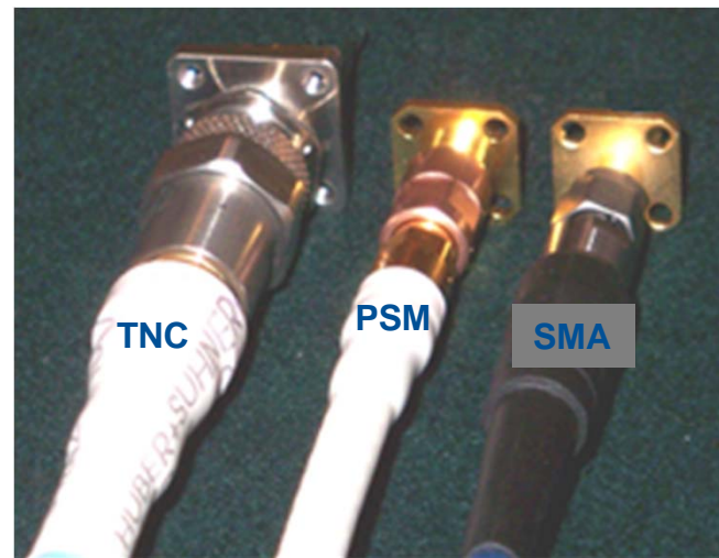
Cable assemblies connected to flange connectors
