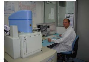
Bond pull and die shear tests Dage series 4000
