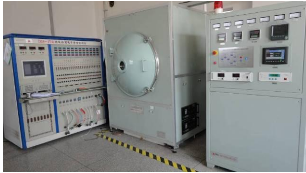
Fig. 1 ZGD-600 ultra high vacuum temperature test chamber
