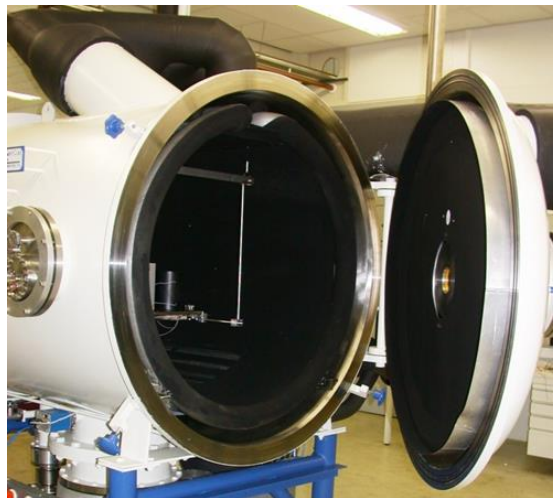
Fig. 3. Photograph of the TV chamber at NLR proposed to be used for the HDTF for space harness designs.
