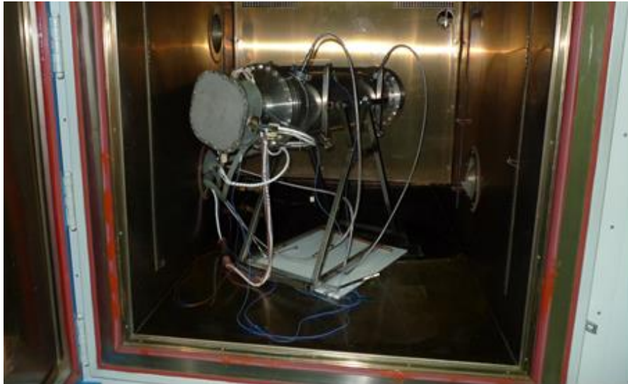
Fig. 1. Photograph of the HDTF for convective environments on a rotatable bench inside NLRs Climate Chamber.
