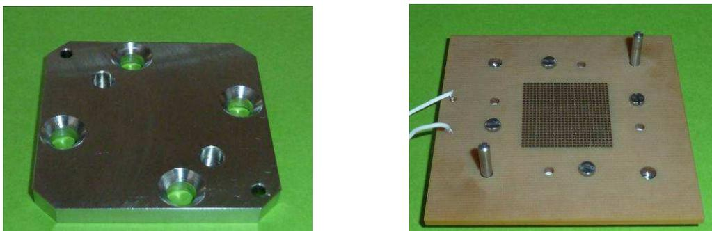
Fig. 7. Additional part used for the adjustment of the PCB (left) and the PCB daisy chain (right)
