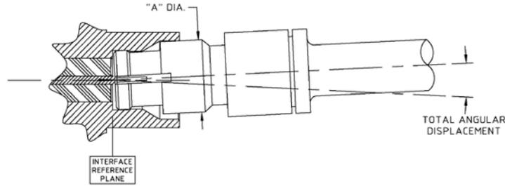
Fig. 2. SMPM interface angular displacement allowance
