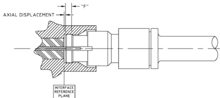
Fig. 1. SMPM interface axial displacement allowance
