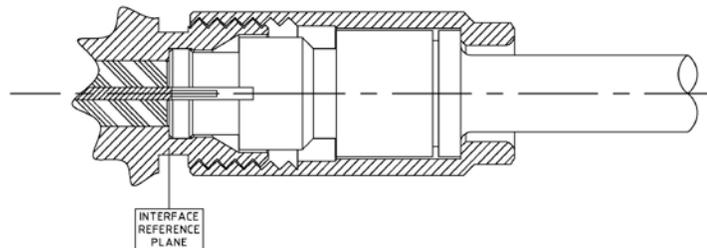
Fig. 3. SMPM-T Male and Female mated connectors
