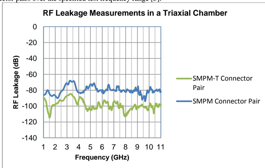
Fig. 5. RF leakage performance of SMPM and SMPM-T connector pairs
