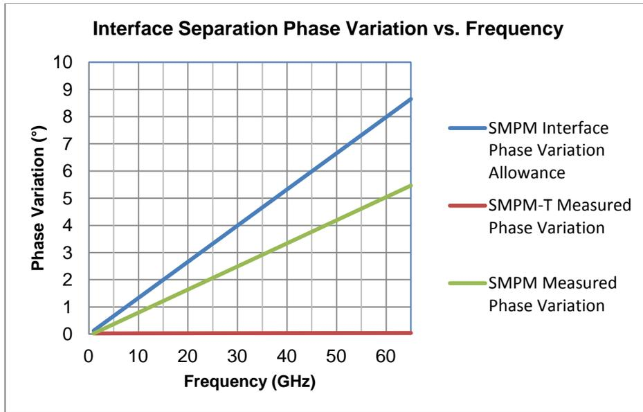
Fig. 4. Interface separation phase impact versus operating frequency
