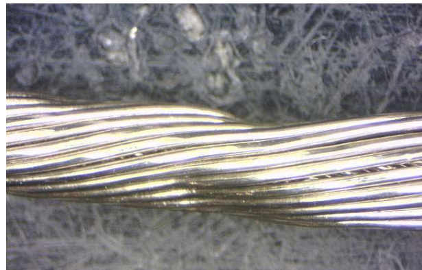
Figure 5. Nickel plated copper conductor aspect after 2000 hours ageing at 250°C.
