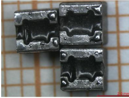
Fig. 3: Typical for inductors; poor solder wetting at solderability test.
