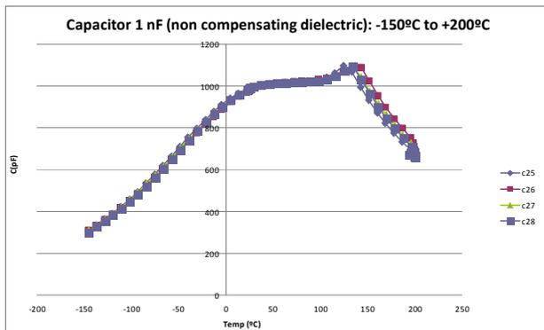
Fig. 10. 1nF standard capacitor
