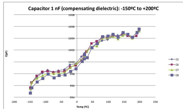
Fig. 11. 1nF temperature compensating capacitor
