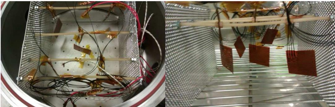
Fig. 12. Heaters in vacuum setup
