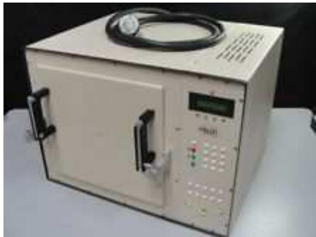
Fig. 1. Sun Systems Climatic Chamber
