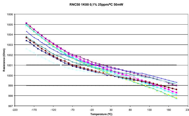
Fig. 6. 1K00 Resistor
