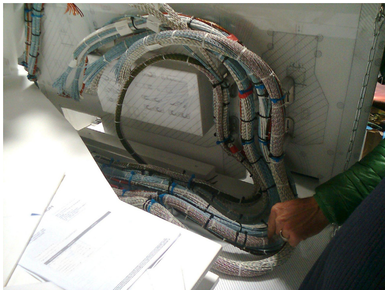
Fig. 2: Detail of the hinge harness mockup on EarthCare Atmospheric Lidar Instrument.
