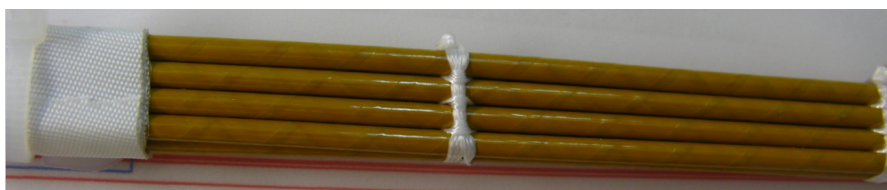
Fig. 6: Flat bundle made of two layers of four AWG12 wires
