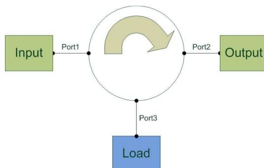
Fig.1. Principle of an isolator
