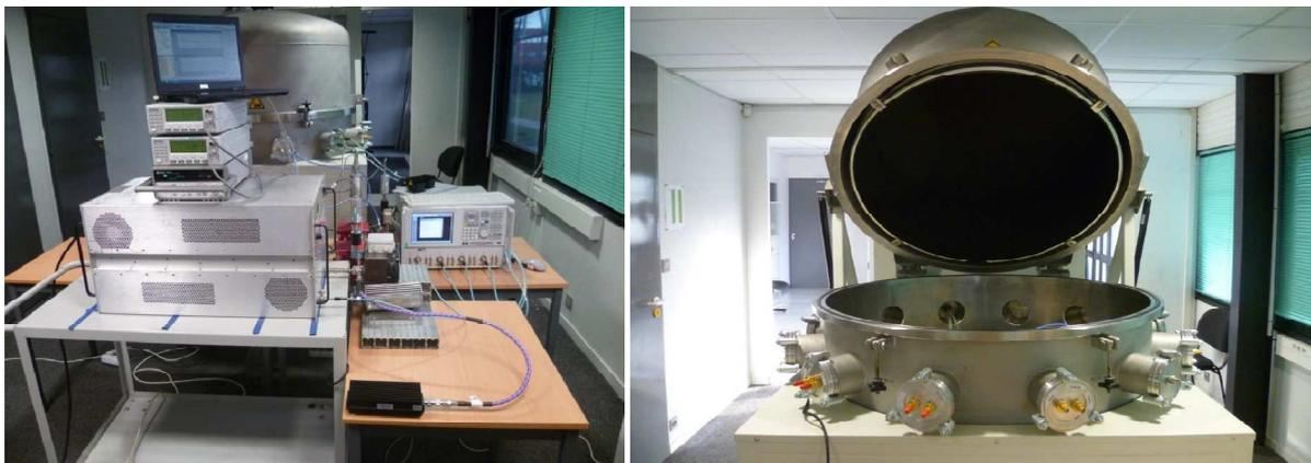
Fig.11 Pictures of thermal vacuum chamber
