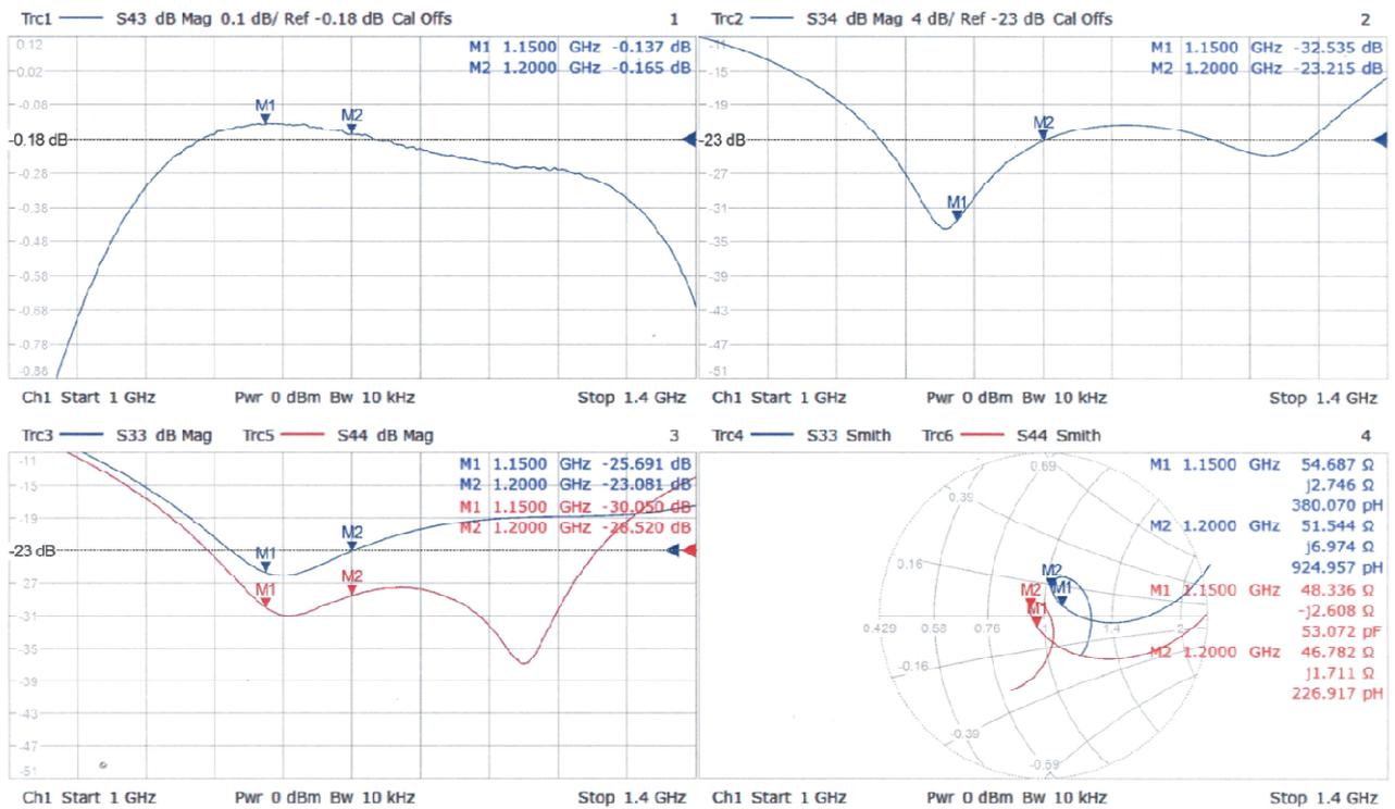
Fig.10 RF measurement after temperature cycling at 25°C
