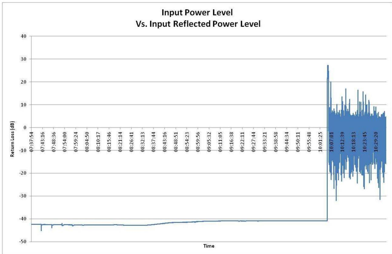
Fig.14 Input power level vs input reflected power level
