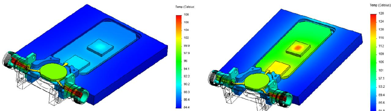
Fig.2. Temperature diagram for 200 W in nominal and short-circuit condition
