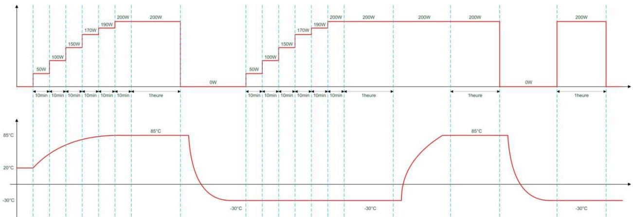
Fig.12 Power handling test sequence
