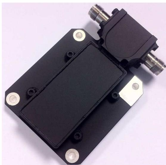
Fig.3. L-band isolator design
