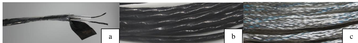
Figure 5: Three cables manufactured in the prototype laboratory - (a) CNT conductor/CNT tape shield; (b) Cu Conductor, CNT tape shield; (c) Cu conductor, Cu braid shield
